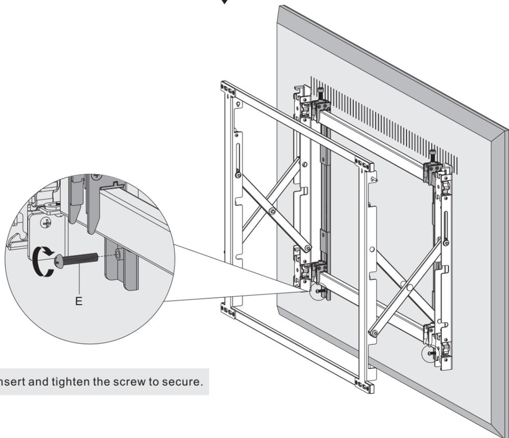
Insert and tighten the screw to secure.
